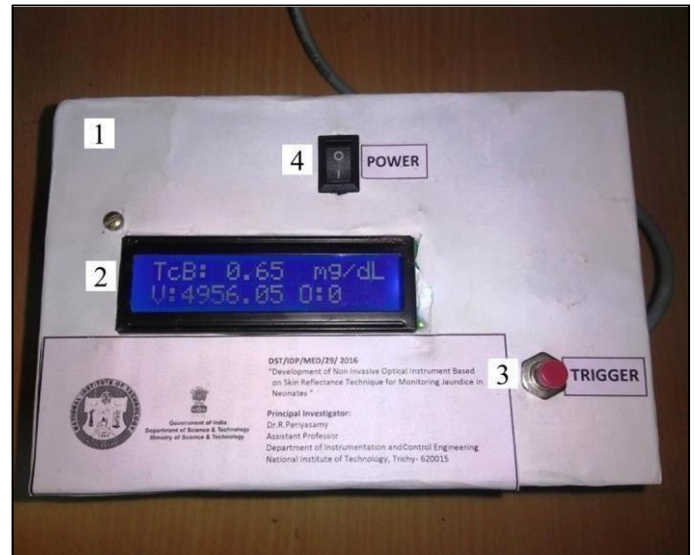
FIGURE 2.4 – (1) CONTROL UNIT; (2) LCD DISPLAY; (3) TRIGGER SWITCH; (4) POWER SWITCH
